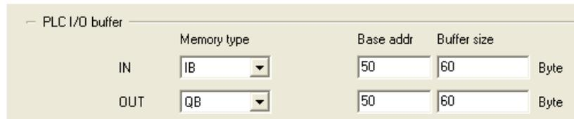
In this example, that is input bytes IB50 to IB 109 (60 bytes) for the TPDOs transmitted by the slave and for the data to be transmitted to the slave (RPDOs) output bytes QB50 to QB 109 (so 60 bytes). These two memory areas are cyclically exchanged by the data handling blocks.
