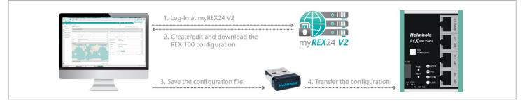
Ensure that the power supply is connected to the REX 100. Download the configuration file provided through the myREX24 portal to the FAT-formatted USB flash drive connected to your PC using the download symbol.
