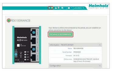
The active connection status to the REX 100 is represented by an animated orange connection button. The number of active connections made using this account is shown with details in the menu bar.
