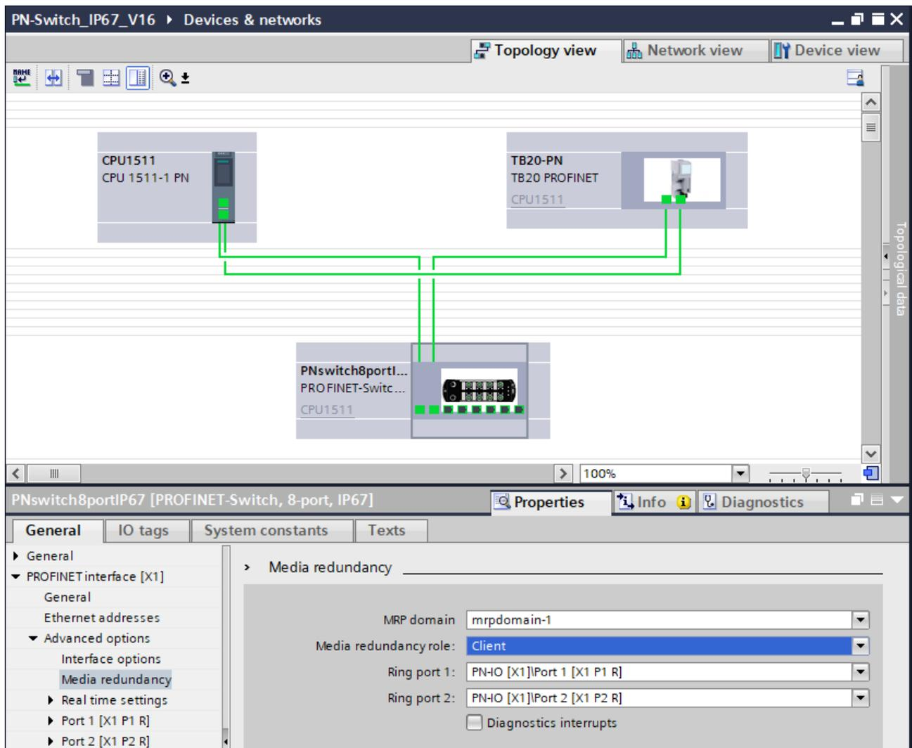
*Important: If ring wiring is established without the MRP roles being configured for all devices involved, this can result in functional disruptions of the PROFINET network!*
