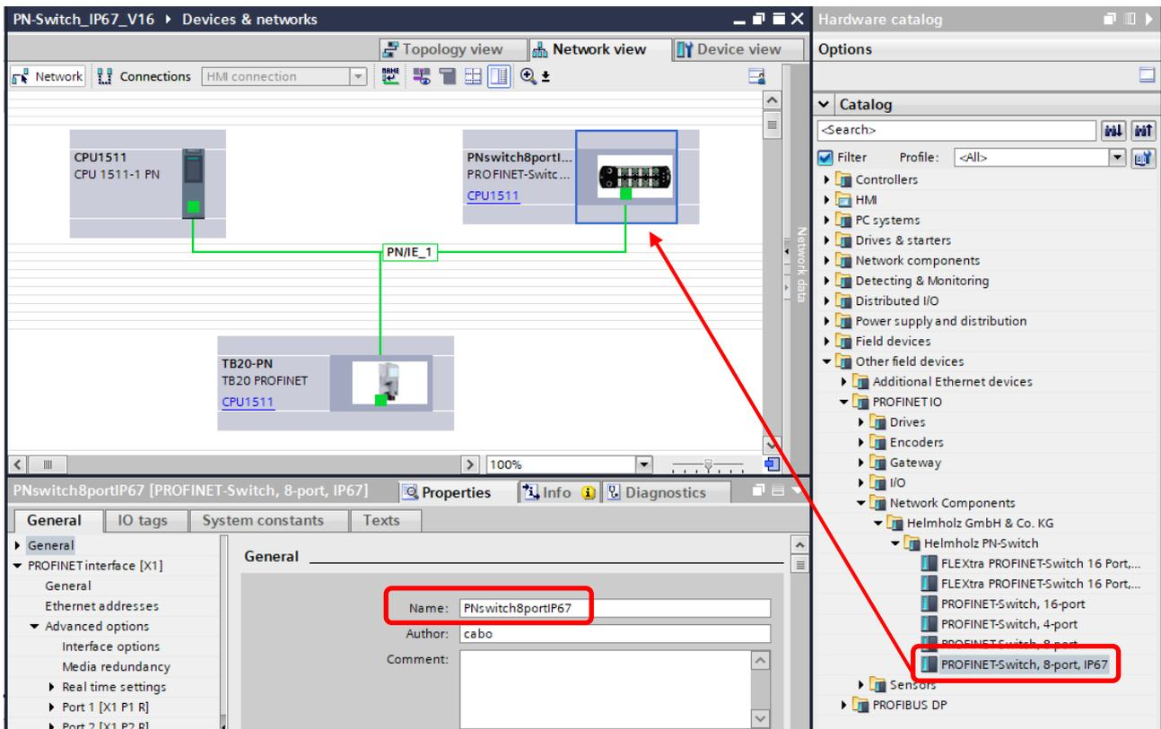
By calling up the device properties, you must assign the PROFINET switch a unique PROFINET name in the project and check the IP address for plausibility.
