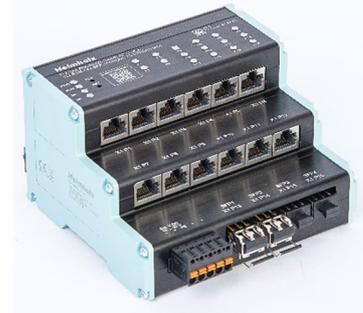
In addition, the FLEXtra PROFINET switches support the control of ports via inputs and the display of port states via outputs. Bits in the PROFINET-IO image of the switch as well as 4 digital inputs and 2 digital outputs with 24V can be used as inputs and outputs. The assignment and the function of the inputs and outputs can be configured via the GSDML file.
