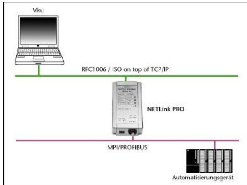
If this ‘RFC1006’ function is activated in NETLink® PRO, explicit adaptations must be made to the software products. This manual describes step by step the basic settings of a small selection of visualization solutions for transferring data via this communication path.
