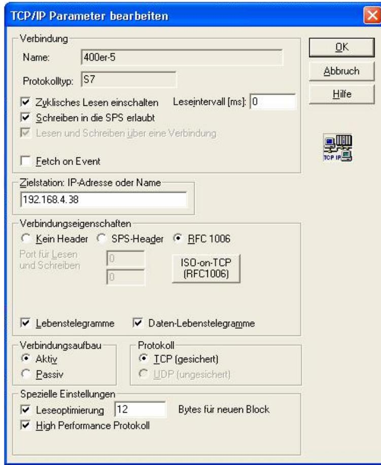
The RFC1006 setting is configured via the “ISO-on-TCP” button.
