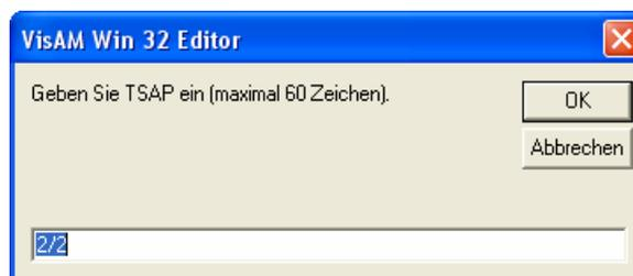
...and enter address. In this case 2/2 for bus address 2, rack 0, slot 2 (see Chapter 10.3.1 -> Address conversion table in NETLink® PRO Manual).
