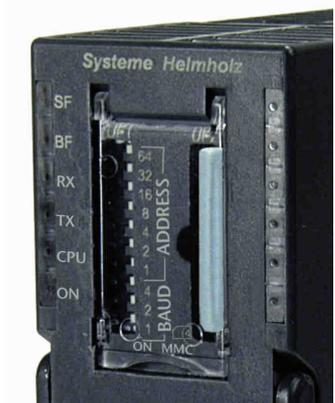
CAN bus reception active: Indicates correct reception of a CAN frame.
