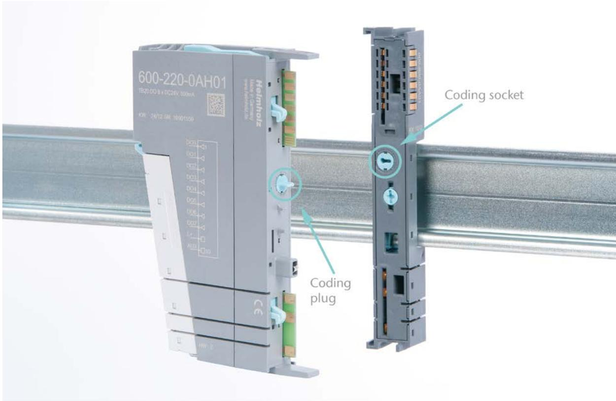
The coding plug and coding socket can each be in one of eight different positions. Each of these eight positions is factory-assigned to a specific type of module (digital in, digital out, analog in, analog out, power, etc.) from the TB20 I/O system. It will only be possible to plug an electronic module into a base module if the position of the coding plug and the position of the coding socket match. Otherwise, the electronic module will be mechanically prevented from being plugged in.
