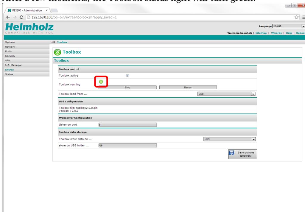
6. As soon as the status light turns green, you will be able to access Toolbox by using the REX router's IP address and the port specified in "Webservice Configuration" > "Listen on port." You can change this port if you need to. However, make sure not to use any of the ports that the REX 300 router is already using for its functions (e.g., 21, 23, 25, 53, 80, 110, 123, 443, 1194, etc.).
