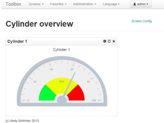
Provided the REX 300 router can reach the PLC, the widget will now refresh the corresponding values and display them after scaling them. You can follow the same basic procedure to add additional widgets to existing or new screens.
