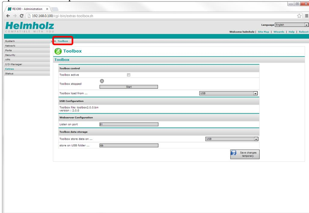
4. Enable the "Toolbox active" check box and click on the "Save changes temporary" button. Then click on the "Apply Changes" button to close the configuration page.
