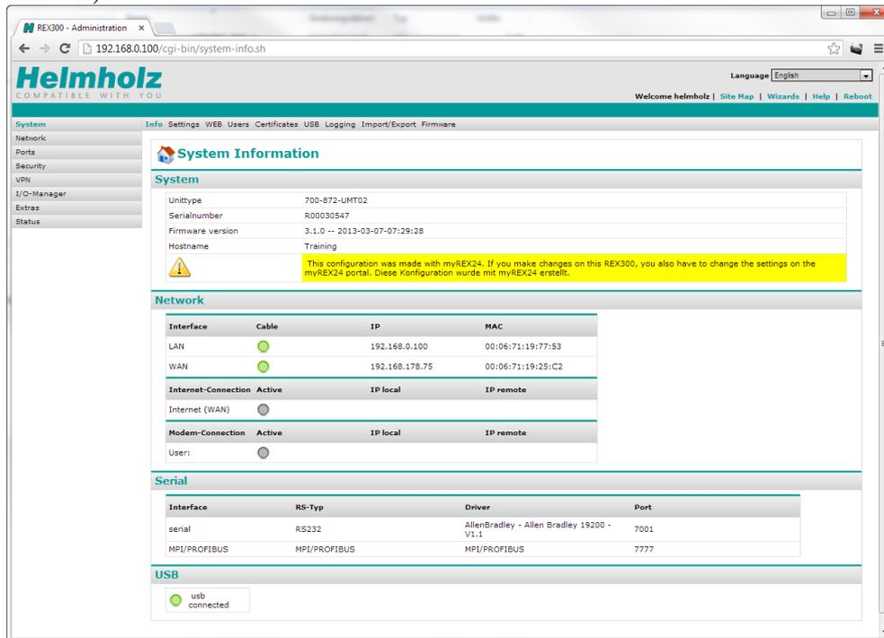
2. Open the "Extras" menu on the left menu bar in order to access the REX 300 unit's special functions.
