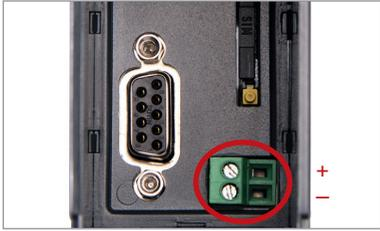
1. First, wire up the REX 300 with a supply voltage of 10-30 VDC.
