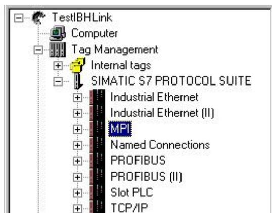
Before you create a controller, the communication parameters must be set. Select menu item "MPI". Now press the right mouse button and select menu item "System Parameter" from the context menu.
