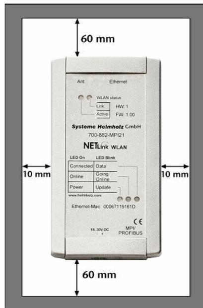
For NETLink WLAN, a minimum clearance of 60 mm must be left above and below and 10 mm at the sides.
