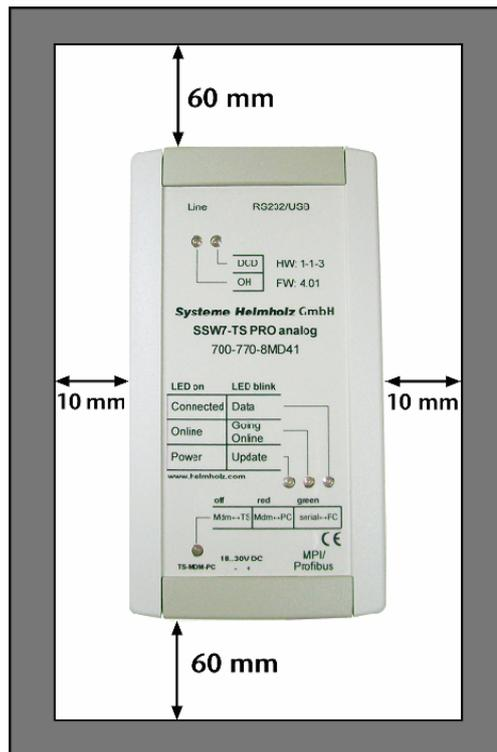
For the SSW7-TS PRO GSM, a minimum clearance of 60 mm must be left above and below and 10 mm at the sides.
