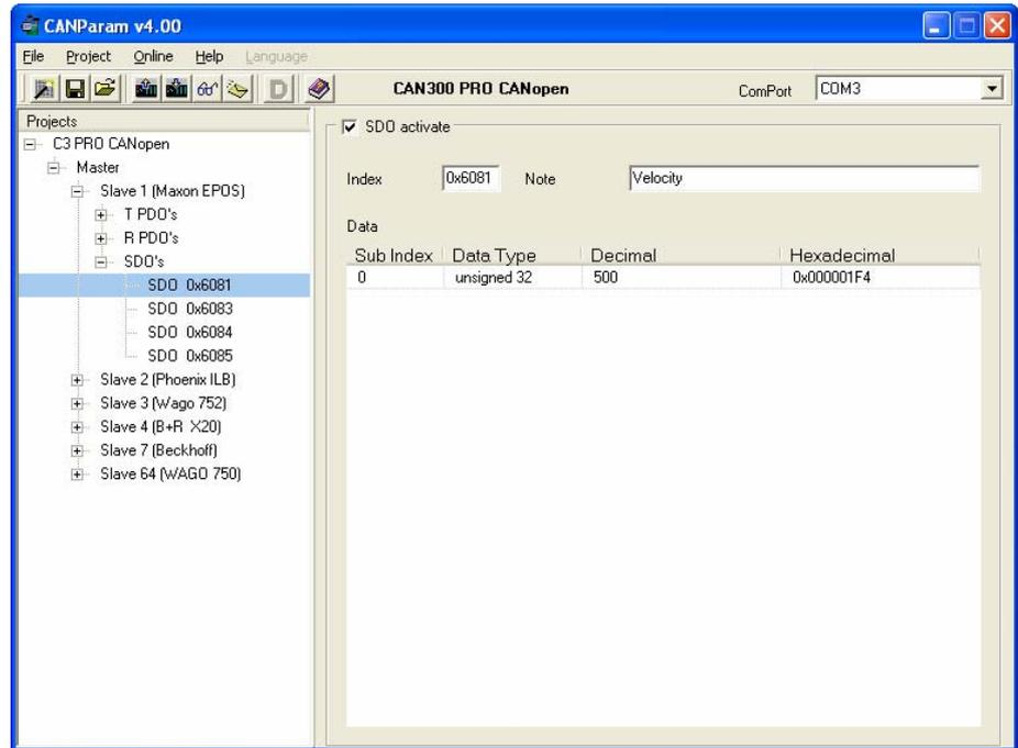
For each slave, a list of SDOs can be stored. The values of these SDOs are written to the slave after start-up of the master and detection of the slave.
