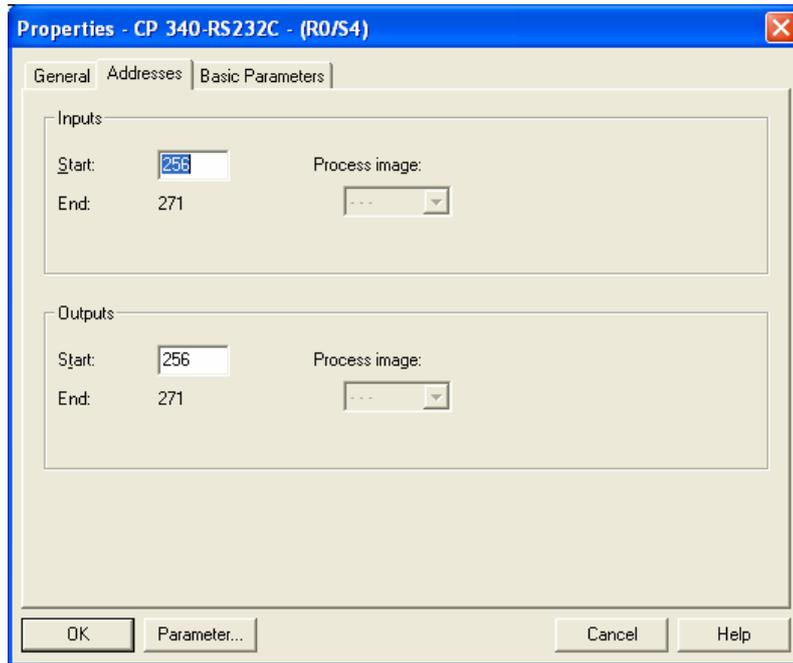
Only the input image is used in the data handling blocks; the output image has no relevance to the function.
