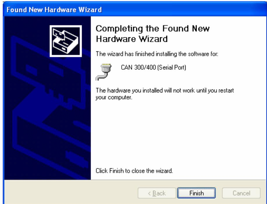
A new COM port has now been added in the device manager. This COM port must be selected in the CANParam software to be able to communicate with the CAN 300 PRO module.
