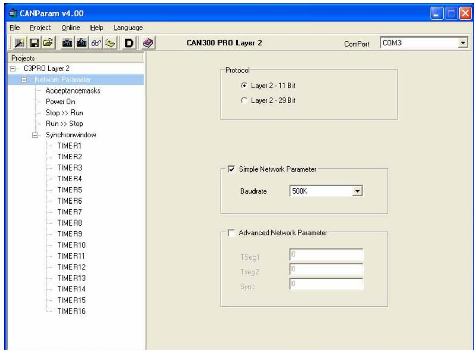
For special applications, you can define the bit time of transmission directly. For a precise description of the bit timing see CAN Specification 2.0 Part B, Section 10 onward.
