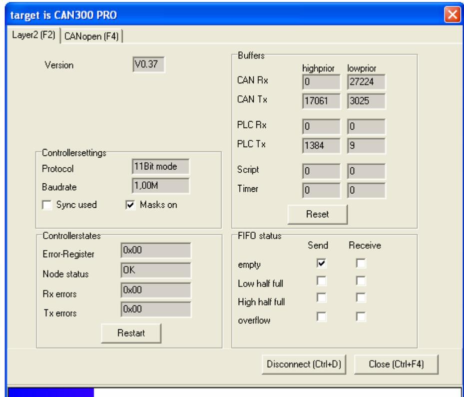
The "Connect" button activates monitoring mode. If you press the button again, the link will be disconnected again.
