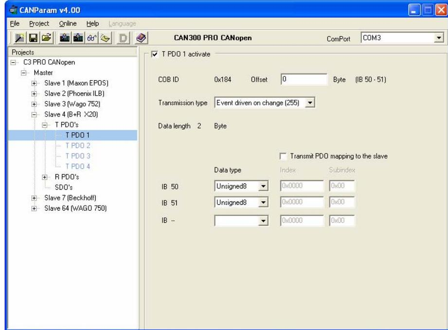
**COB-ID:** Display of the associated CAN-ID. This can not be adjusted and is calculated depending on the node ID and the PDO number.
