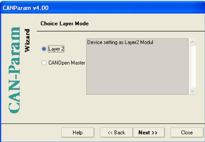
The screenshot shows the 'Choice Layer Mode' dialog box. On the left is the 'CAN-Param Wizard' logo. Two radio buttons are visible: 'Layer 2' (which is selected) and 'CANopen Master'. To the right of the 'Layer 2' option is a text box containing the text 'Device setting as Layer2 Modul'. At the bottom are the 'Help', '<< Back', 'Next >>', and 'Close' buttons.
