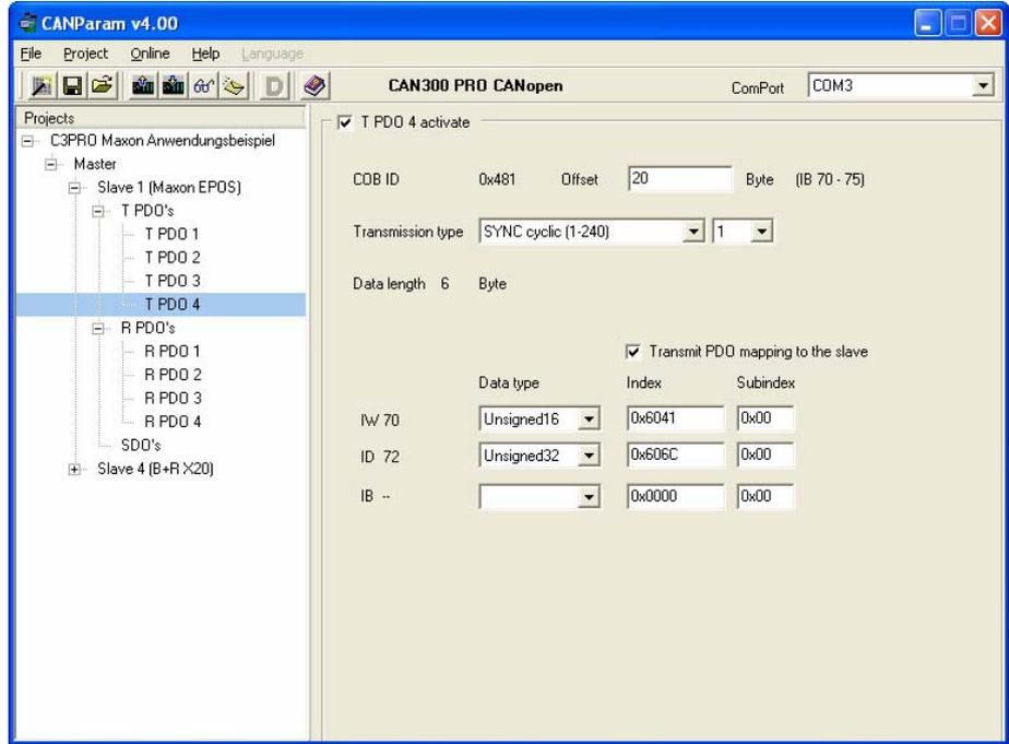
In the PLC, the value of SDO 6041 in IW 70 can now be processed and the value SDO 606C is in ID 72. The values are automatically adapted to the data format of the PLC.
