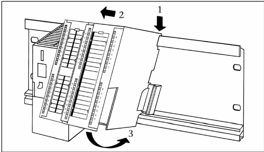
Screw the modules on with a torque of 0.8 to 1.1 Nm.
