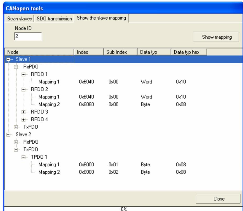
**Node ID:** Node-ID of the slave, which PDO mapping data will be fetched.
