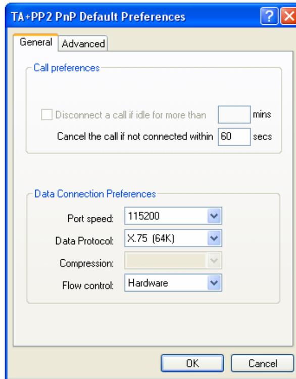
“X.75” is the standard protocol for data transmission in packet switched ISDN networks with a transmission rate of 64 kbps.
