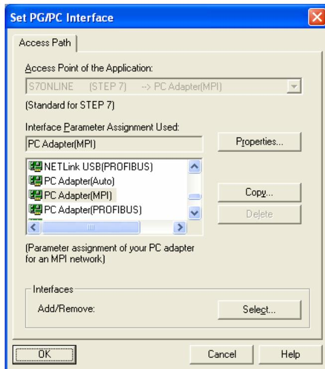
Under the "Properties" of the MPI or Profibus settings, the appropriate COM port must be selected before first use. On connection via USB, the previously installed virtual COM Port must be set (see Section 4.2).
