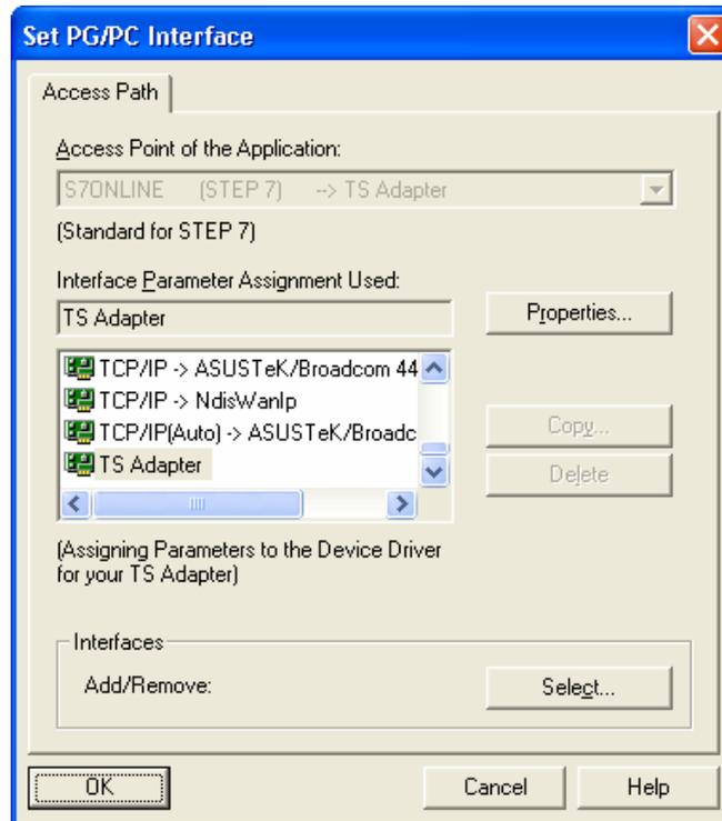
For teleservice, the “Modem connection” mode must be selected on the “Local connection” tab card in the properties of the TS adapter.
