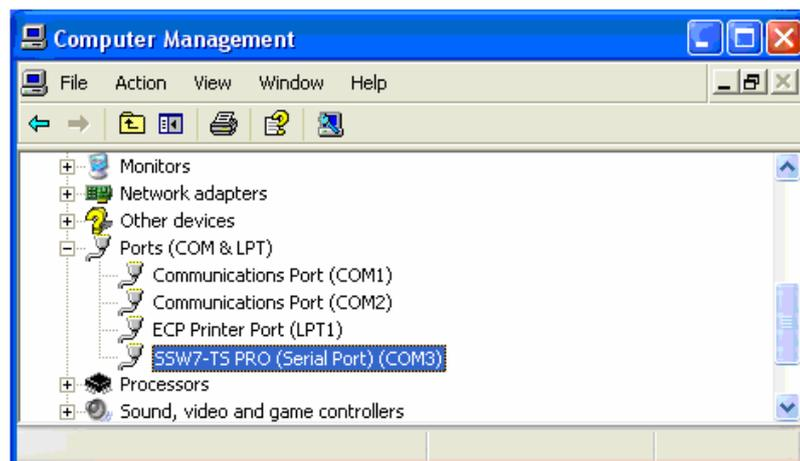
If several USB interfaces are available, but the SSW7-Teleservice-Modem CD is not at hand, we recommend copying the driver files onto the local hard disk because it is possible that a separate instance of the driver for the SSW7-TS PRO ISDN has to be installed on the PC for each USB interface.
