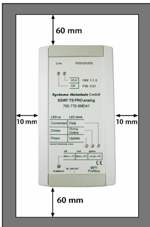
For the SSW7-TS PRO analog, a minimum clearance of 60 mm must be left above and below and 10 mm at the sides.
