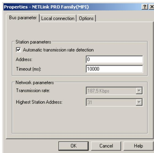
The most important setting concerning bus configuration is assignment of the station address. This refers to the address the NETLink® PRO PoE will have on the bus when it goes online.
