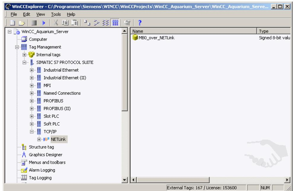
If this variable is now included in the initial screen of the WinCC project, for example, a connection will be established to the CPU with address 49 via the NETLink® PRO PoE to read or write marker byte 0 from this rack 0, slot 2.
