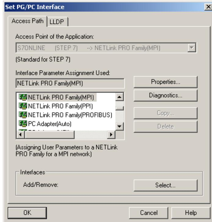
All relevant settings of a NETLink-S7-NET driver can be made via the 'Properties' access field. With the button 'Diagnostics...', it is possible to show the nodes connected to the bus and the parameters the bus is working with. These fields are explained in Section 5.
