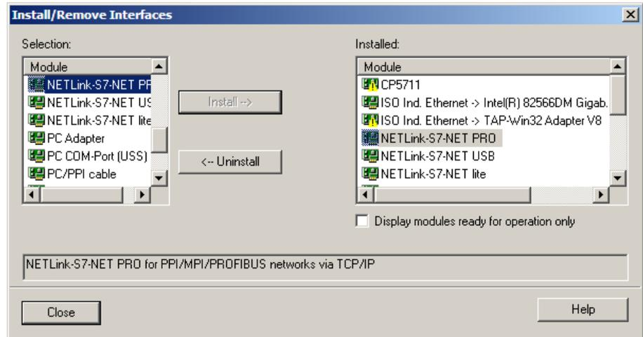
The access path in the 'Set PG/PC Interface' dialog box is set when this window is closed.
