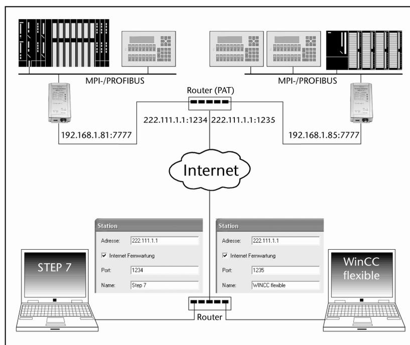
By default, the S7 network driver attempts to address the NETLink<sup>®</sup> PRO PoE via fixed port 7777, which would not work in the above scenario.
