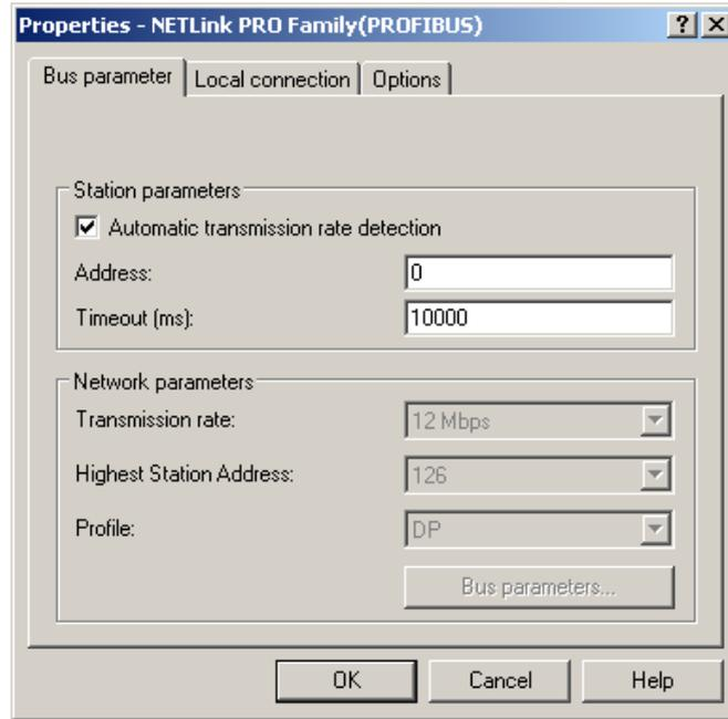
Under PROFIBUS, please note that the auto baud function works best if the 'Cyclic distribution of the bus parameters' function is activated in the programmable controller used.
