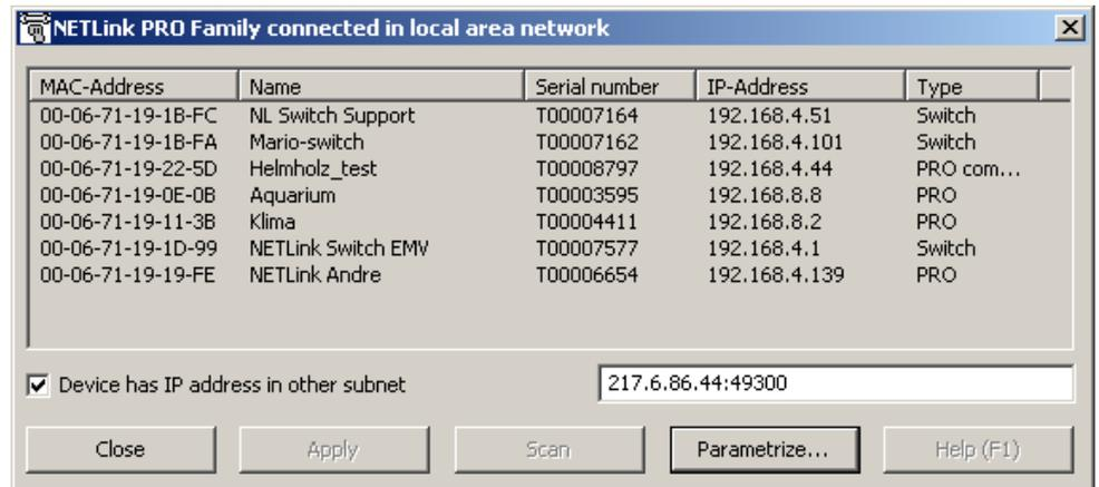
An extended function enables direct parameterization across network boundaries. To do this, activate the radio button and enter the known IP address of the NETLink® (the example includes the optional address of the port – separated by a colon) in the empty field. The corresponding configuration menu then opens when "Parameterize..." is clicked.
