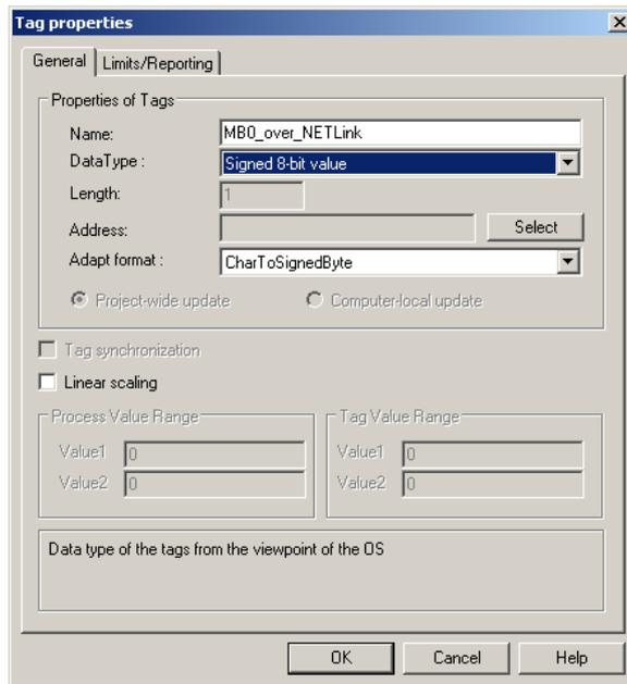
In the properties window of the variable, which was named 'MBO\_over\_NETLink' in this case, we can now select the type of variable by clicking the 'Select' button.
