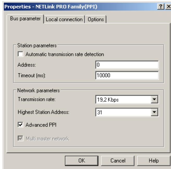
In addition to the parameters transmission rate and highest station address mentioned in Section 5.1.1, PROFIBUS also has a parameter field for selecting the bus profile and bus parameters:
