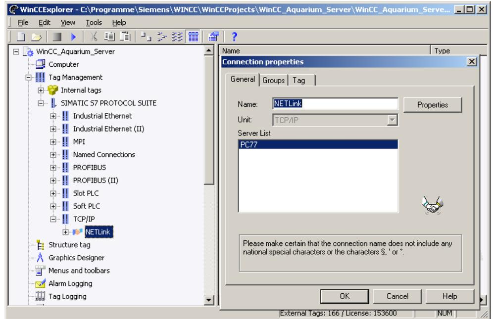
A click on 'Properties' takes us to a setting form in which the IP address of the NETLink<sup>®</sup> PRO PoE and the rack/slot combination of the destination have to be entered.
