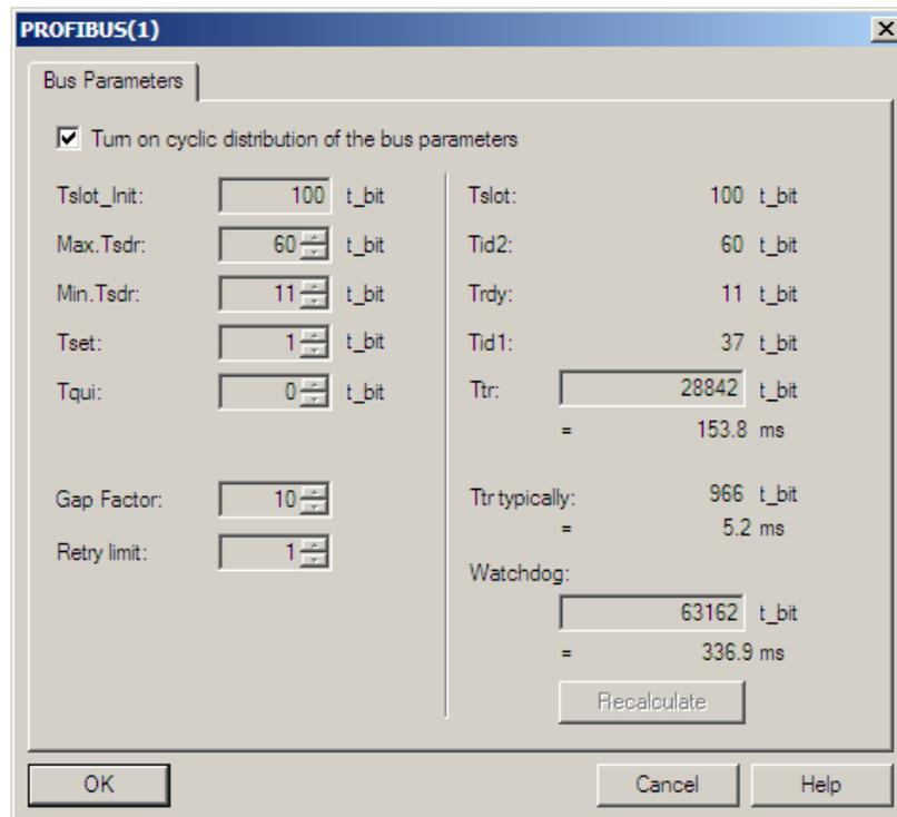
The screenshot above of a hardware configuration of a randomly chosen PROFIBUS CPU shows where to find the switch for cyclic distribution of the bus parameters.
