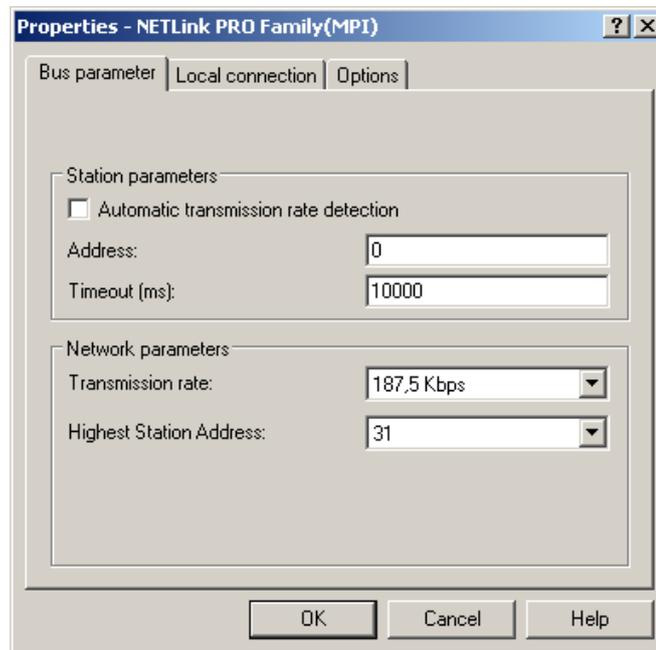
The transmission speed and the HSA of the PLC being addressed must be known and identical to all connected bus nodes.
